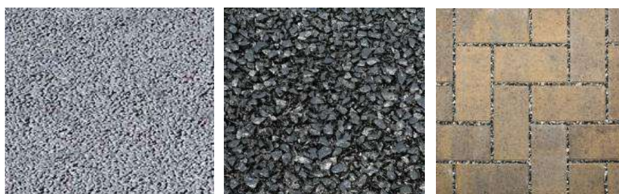
Figure 58. Porous concrete, porous asphalt and interlocking pavers
