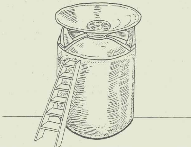
Figure 7 A Freestanding Cistern with a Conical Collecting Roof.
