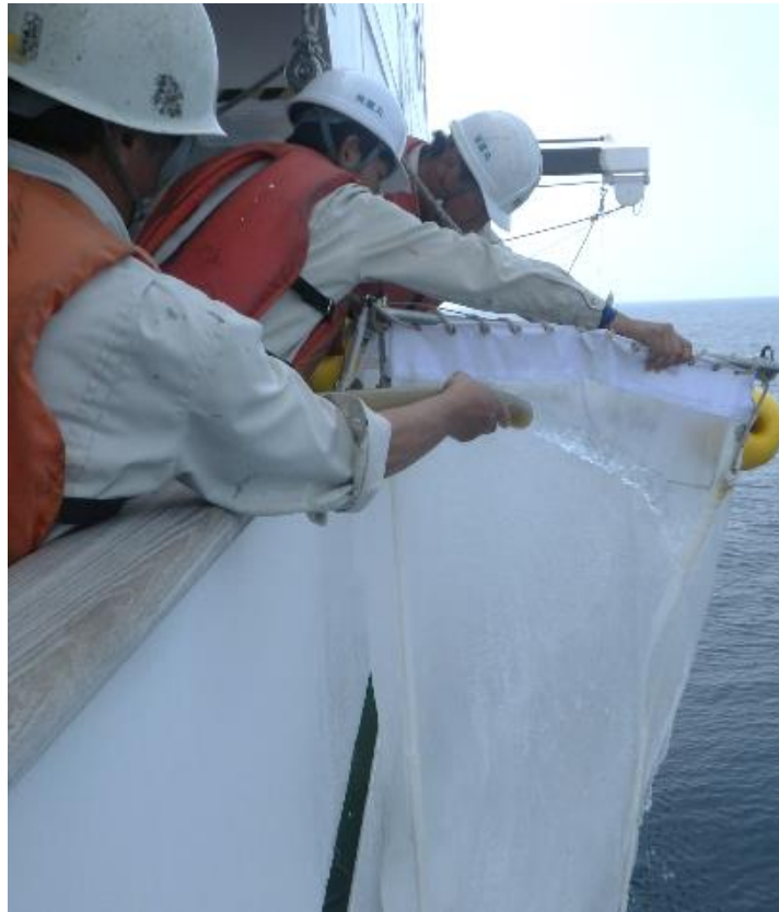
Wash away sticking sample to codend
