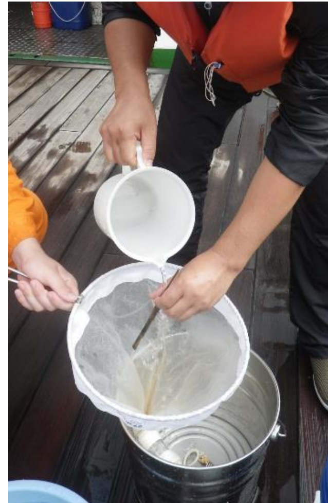
Remove large debris after wash away small litters
