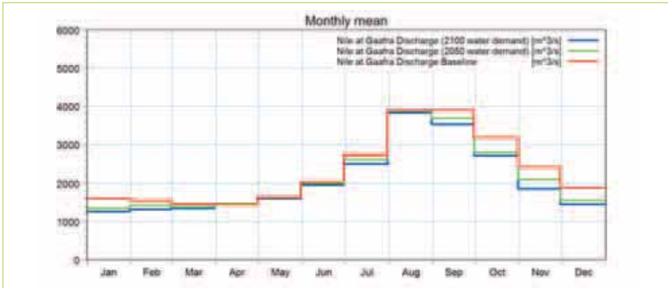
Figure 8.5 Mean monthly discharges for the Gaafra (El-Ga'Afra) gauge for baseline, 2050 & 2100 water demands
