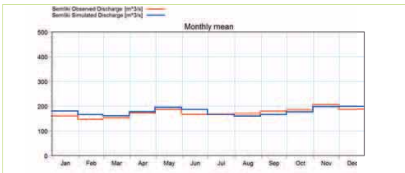
Figure 5.52 Comparison of the observed (red) & simulated (blue) mean monthly flows at the Semliki station for the period 1960-1980
