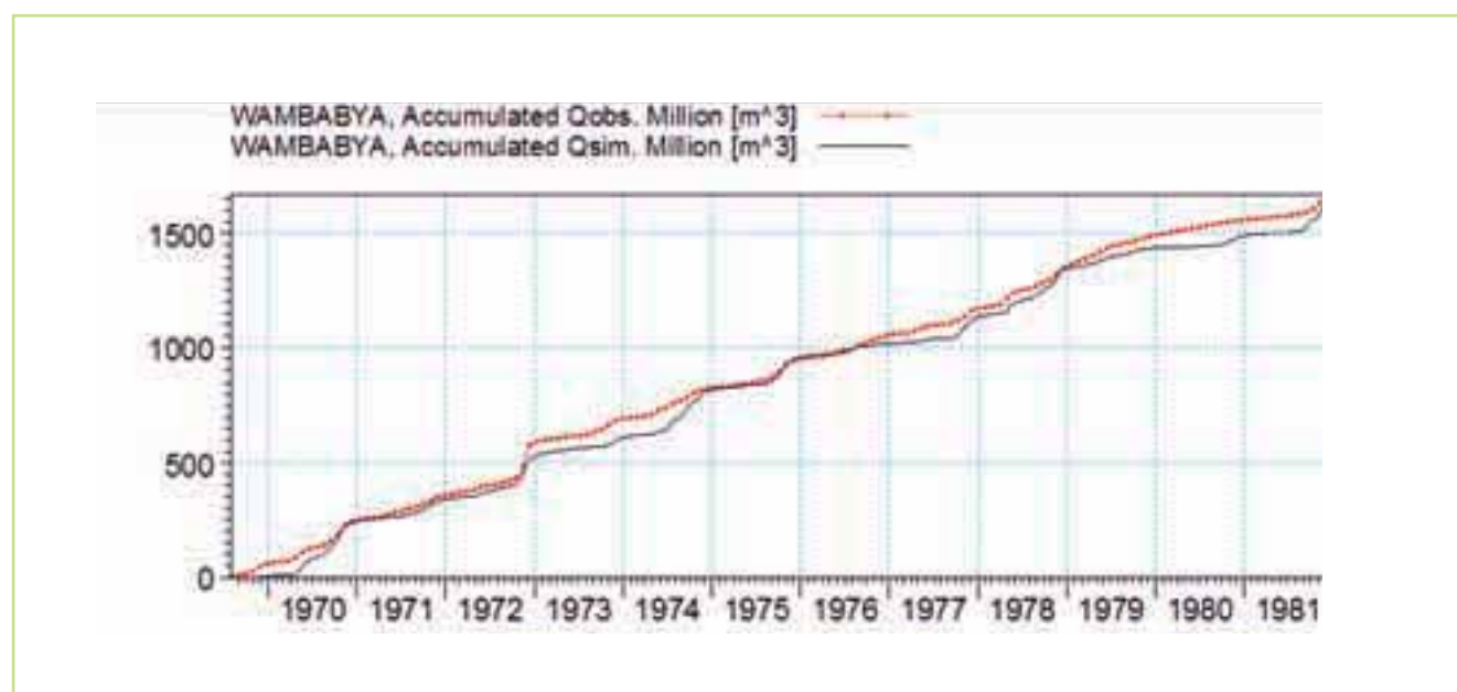
Figure 5.11 Example of accumulated mass curves for the observed (red) and simulated (black) discharge for the Wambabya catchment. There is a reasonable agreement between the two hydrographs with the exception of 1980 where the observed data is probably not reliable
