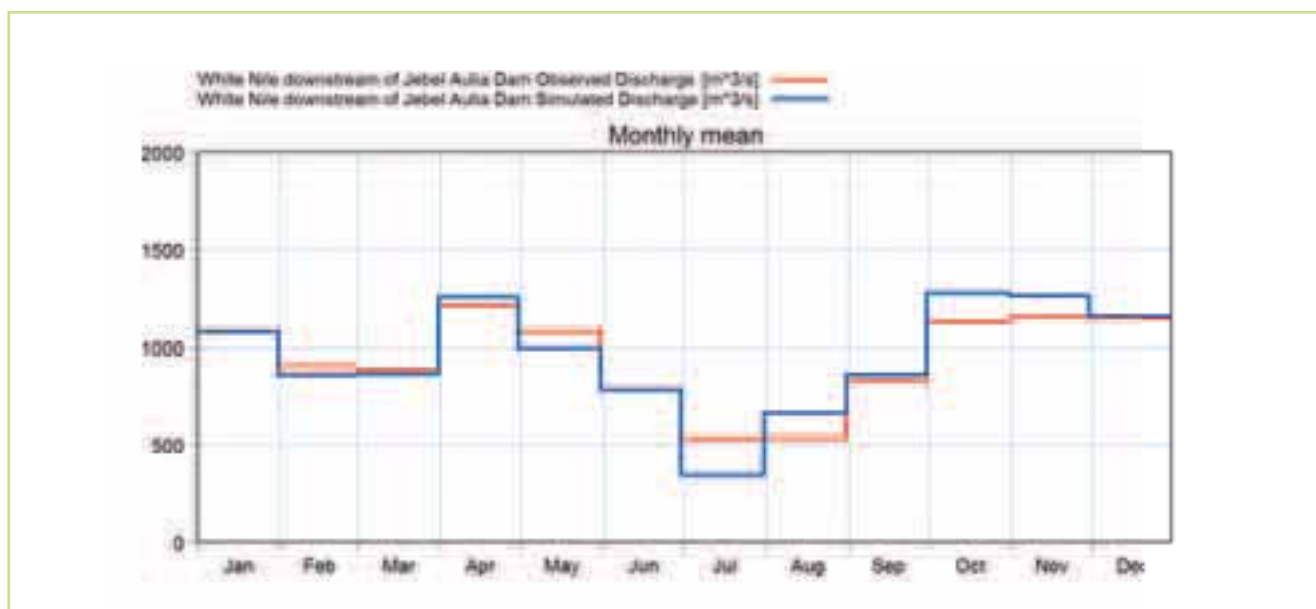
Figure 5.78 Comparison of the observed (red) & simulated (blue) mean monthly flows at the Jebel Aulia station for the period 1960-1980.
