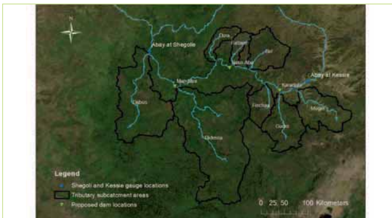
Figure 5.45 Tributary catchment areas & proposed dam locations between the Shegoli and Kessie gauges
