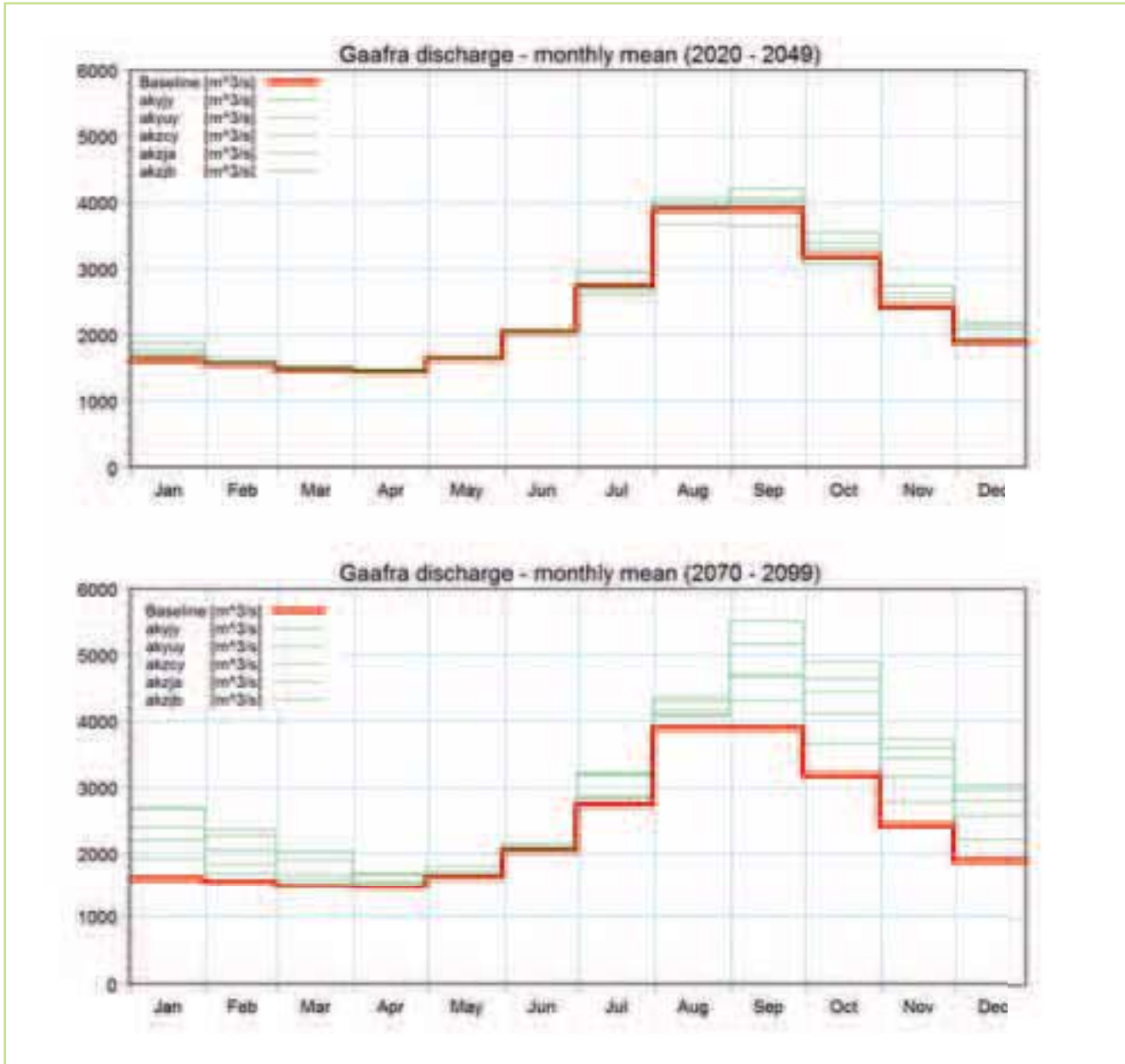
Figure 8.6 Projected changes in the average monthly flows for the Gaafra (El-Ga'Afra) station for the two periods; 2020-2049 & 2070-2099. The solid (red) line shows the baseline levels (1961-1990) & the thin green lines the different RCM ensemble members.
