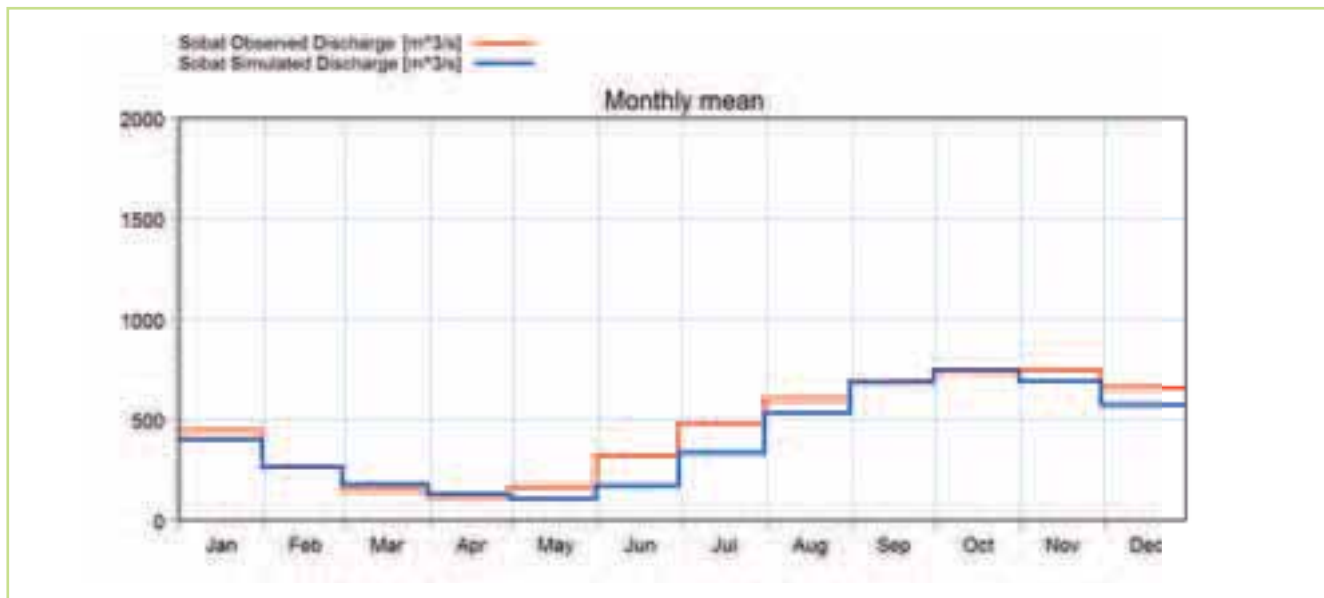
Figure 5.71 Comparison of the observed (red) & simulated (blue) mean monthly flows at the Sobat station for the period 1960-1980
