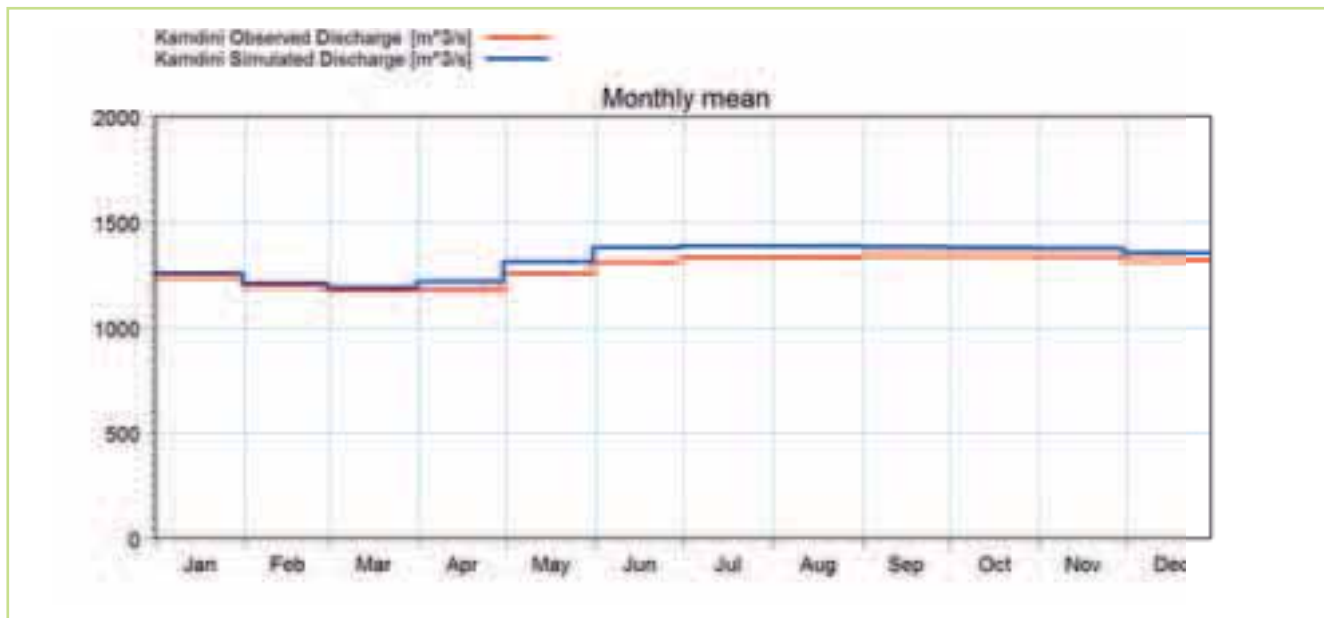
Figure 5.62 Comparison of the observed (red) & simulated (blue) mean monthly flows at the Kamdini station for the period 1960-1980
