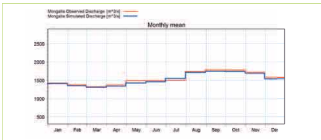
Figure 5.65 Comparison of the observed (red) & simulated (blue) mean monthly flows at the Mongalla station for the period 1960-1980
