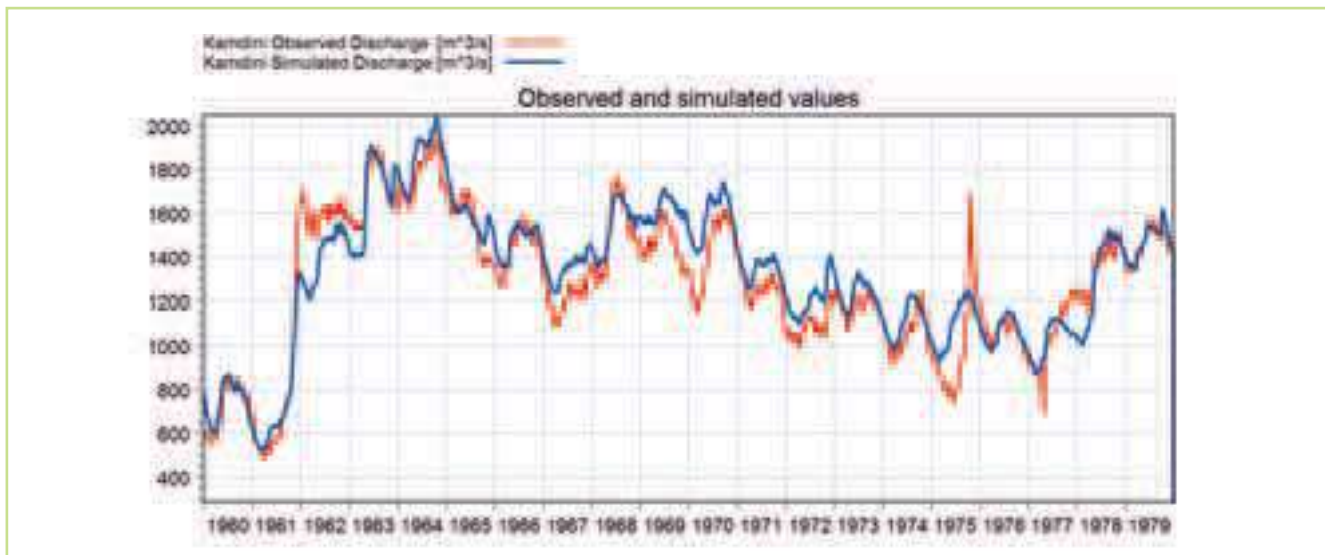
Figure 5.21 Comparison between observed (red) & simulated (blue) discharge at Kamdini (83206) for the modelling period 1960-80
