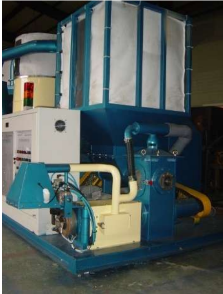
Fig 7. Injection molder (30 kg/hour).
