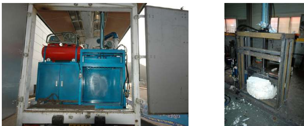
Fig 3. Hydraulic cutter for large buoy.
