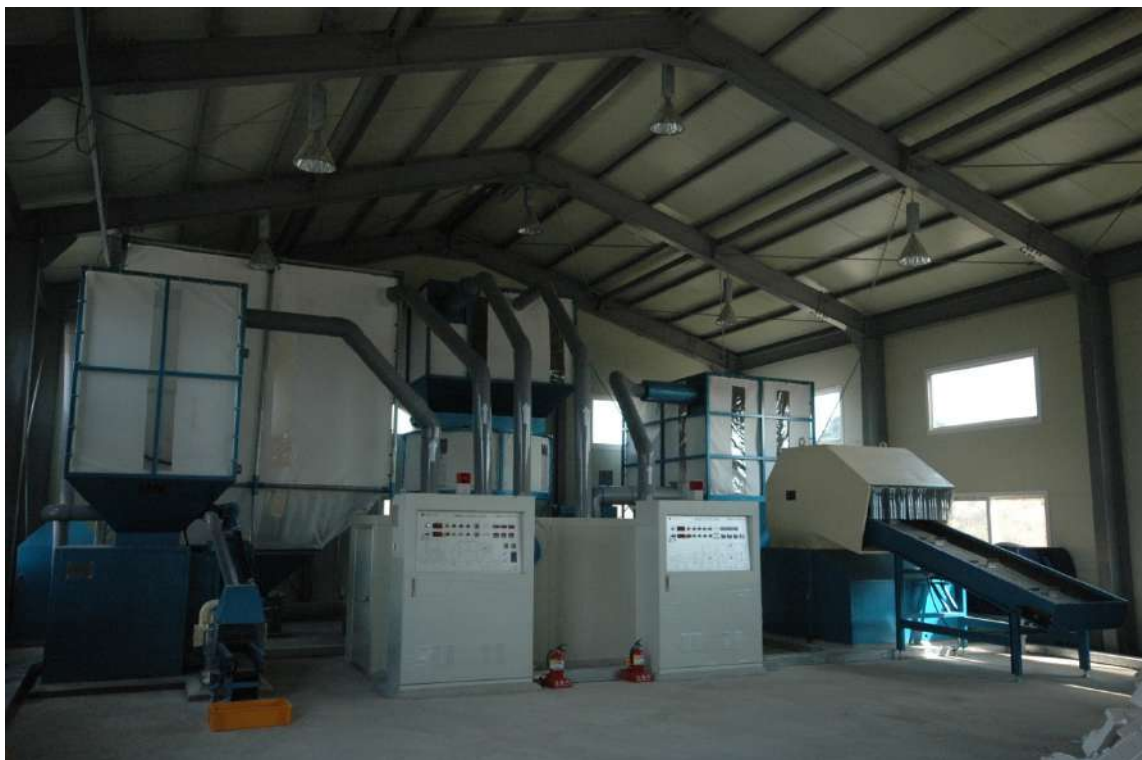
Fig 2. Used polystyrene buoy thermal volume reduction system.
