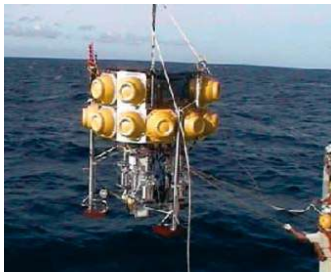
Figure 6.24 Experimental chamber going to the sea floor (Ishida et al. 2004). The bottom part houses a chamber that penetrates into the sediment. The top part houses electronics, pumps, valves, and water bags, that are used to control the CO 2 concentration inside the chamber, and to sample sea water in the chamber at designated times. At the time of recovery, the bottom of the chamber is closed, weights are released, and the system returns to the surface of the ocean using buoyancy provided by the glass bulbs (yellow structures around the top).
