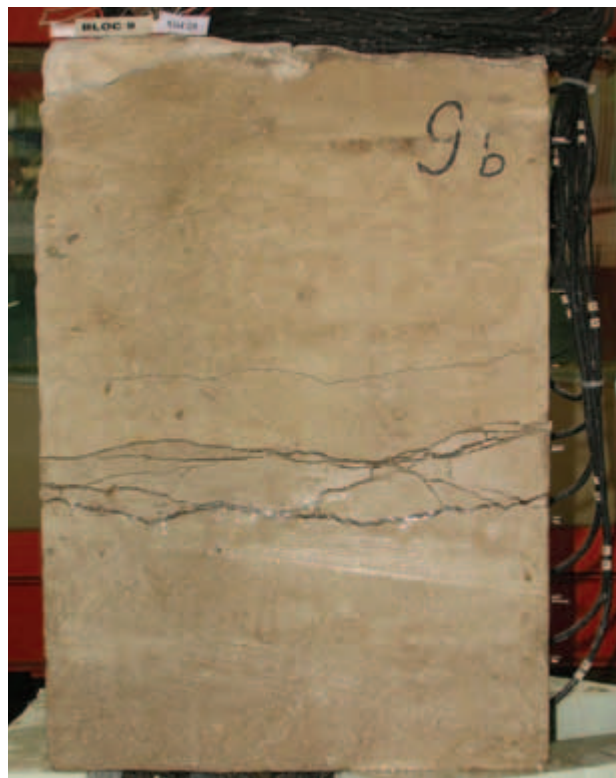
Figure 5.23. Fractures formed by ice segregation in Totternhoe Stone (a type of English chalk) following twenty-four cycles of bidirectional freezing of an active layer above permafrost. The fractures are filled with segregated ice and occur primarily in near-surface permafrost and at the base of the active layer. Some narrow cracks are also visible in the upper part of the active layer, caused by downward freezing from the rock surface. The block is 450 mm high and 300 mm wide. Photo Julian Murton, University of Sussex, UK.
