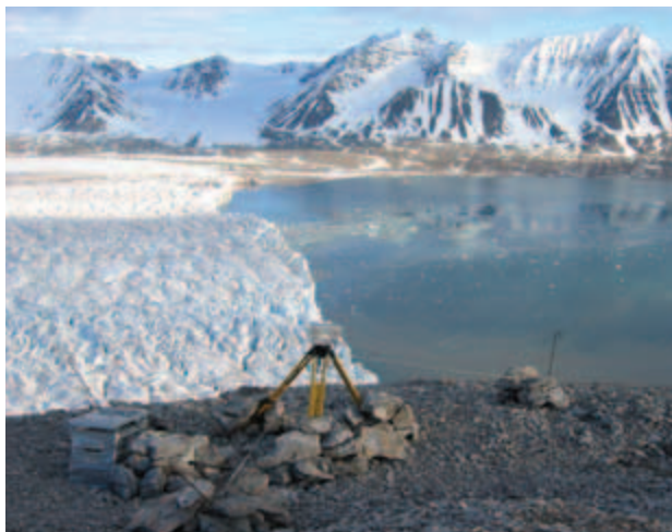
Figure 7.5. Time-lapse camera overlooking the calving terminus of the tidewater glacier, Kronebreen, in Svalbard. Kronebreen is a focus of study within the IPY GLACIODYN project. Source: Monica Sund, University Centre, Svalbard.
