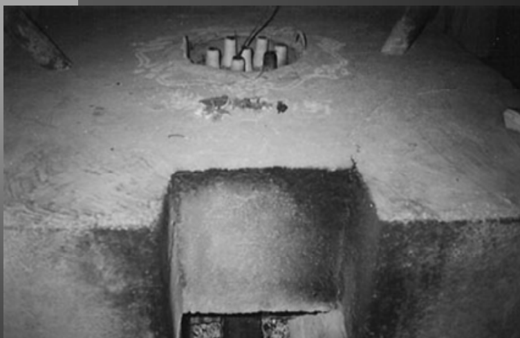
Bottles in furnace coated with multani murti and filled with mercury and sulfur
