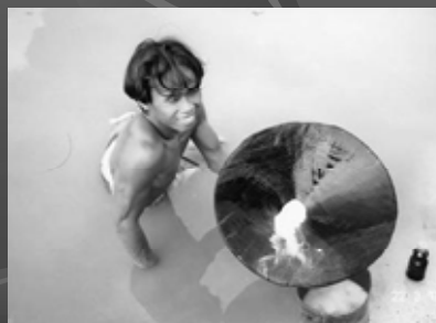
Using liquid Hg to amalgamate gold
