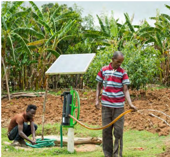
Using a solar-powered water pump to pump groundwater for irrigation in Ethiopia ( Maheder Haileselassie/IWMI )
