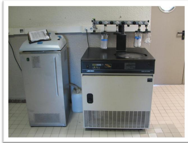
Laboratory device for lyophilization
