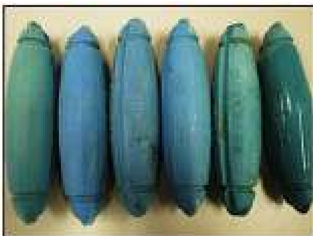
Figure 18. PVC fishery floats with high concentration of Pb.
