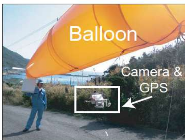
Figure 14. Balloon photography system to monitor distribution of marine litter in Japan.
