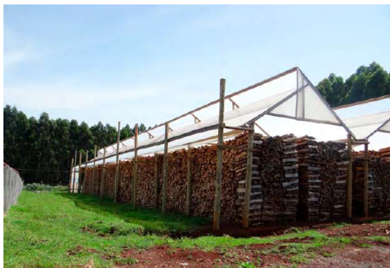
FIGURE 19: Wood drying before use in a boiler fed by woody biomass at Finlays estate (Kericho)
