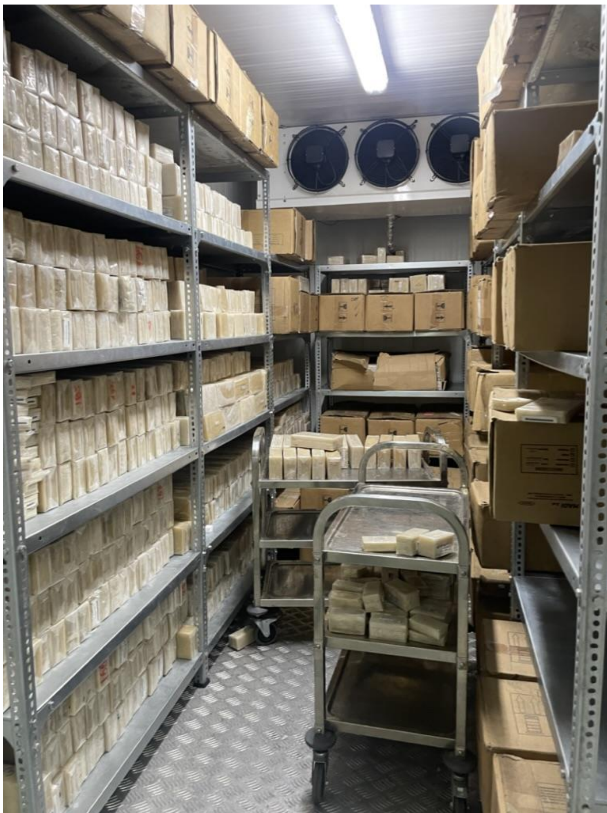
Figure 4 Blocks that simulate food inside refrigerators in testing chambers in a testing laboratory in Santiago, Chile, 13/JAN/2023
