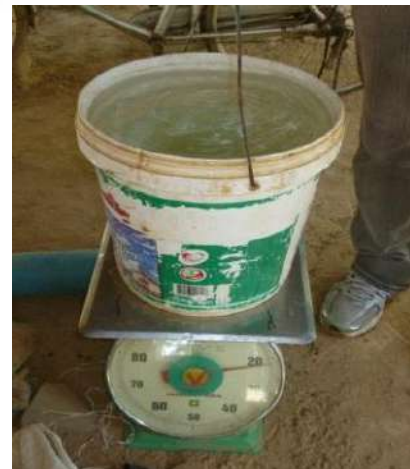
Cow dung feedstock : daily feedstock is 10-15 kg./day >> 4 to 6 cubic meters; stove: 2-4 hours; lighting 8 hours.
