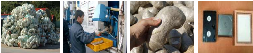
Figure 14. Use of a mobile type of volume reduction system/ a truck mounted mobile system compressor in Korea (Korea Research Institute of Ships and Ocean Engineering).
