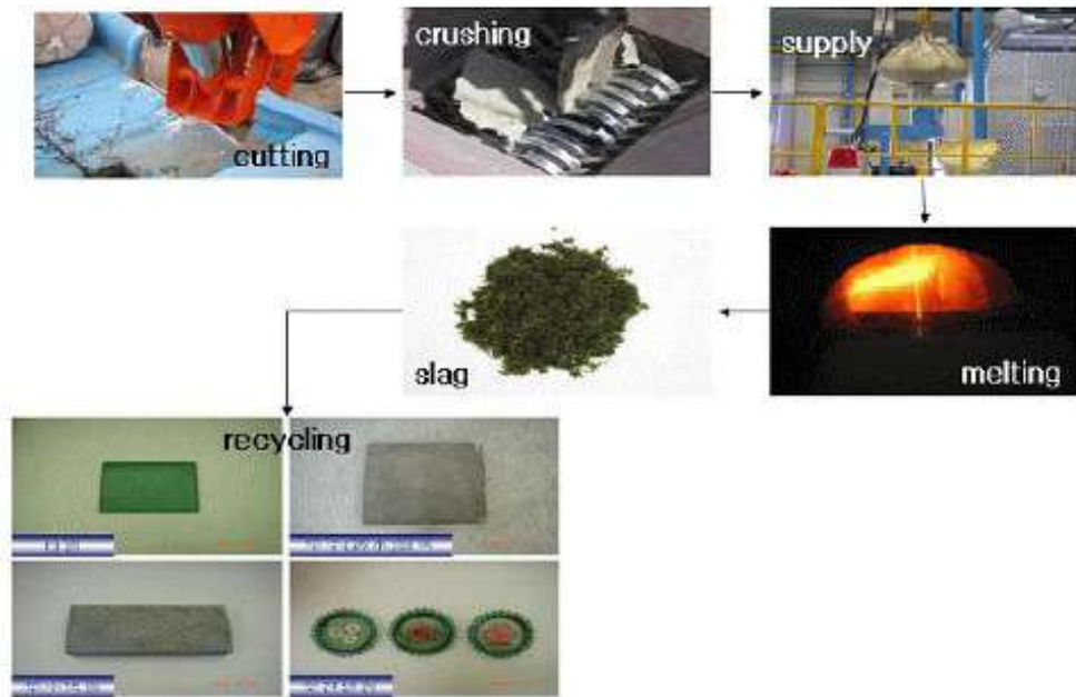
Figure 19. Process of waste FRP vessel melting treatment (MERRAC, 2010).
