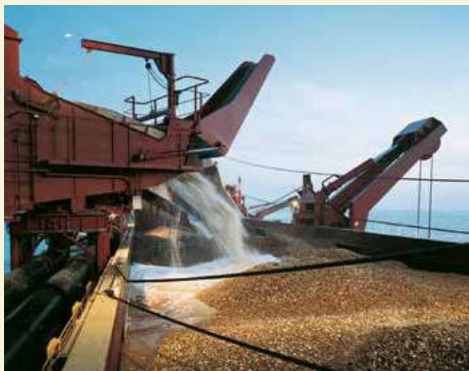
2.8 > A suction dredger extracts sand from the North Sea floor off the Dutch island of Ameland to widen the beach.
