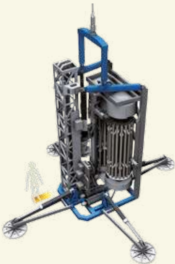
3.10 > The underwater rig MARUM-MeBo has been used for several years for drilling on the sea floor. It is flexible in that it can be deployed from different research vessels. Methane hydrate could be mined in the future using similar equipment.
