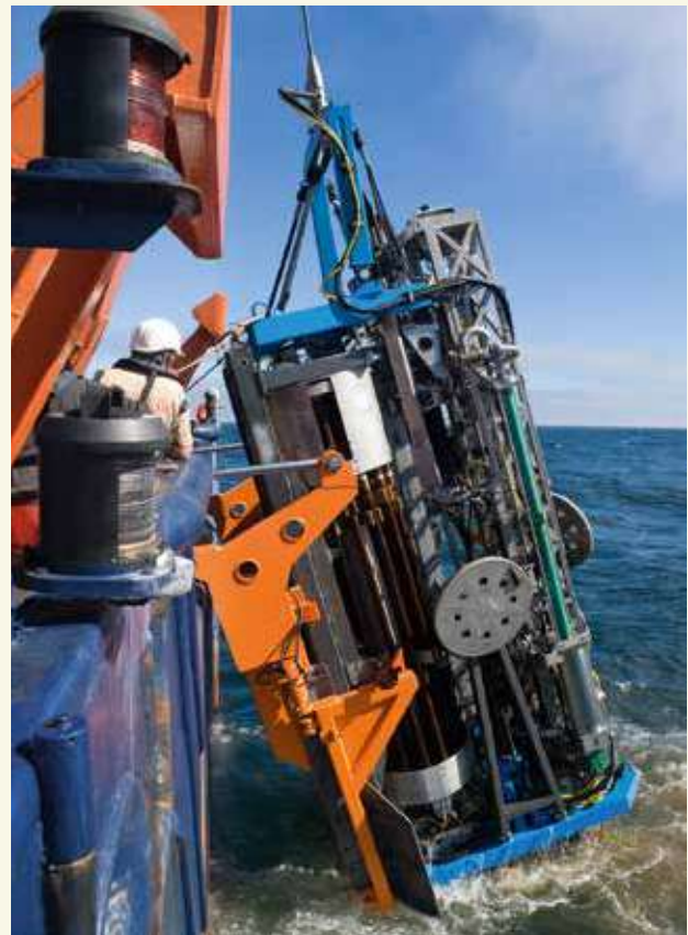
3.10 > The underwater rig MARUM-MeBo has been used for several years for drilling on the sea floor. It is flexible in that it can be deployed from different research vessels. Methane hydrate could be mined in the future using similar equipment.
