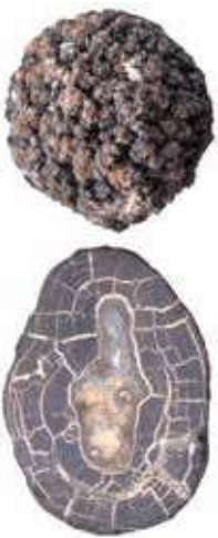
2.10 > Slice through a manganese nodule: Over millions of years minerals are deposited around a core.
