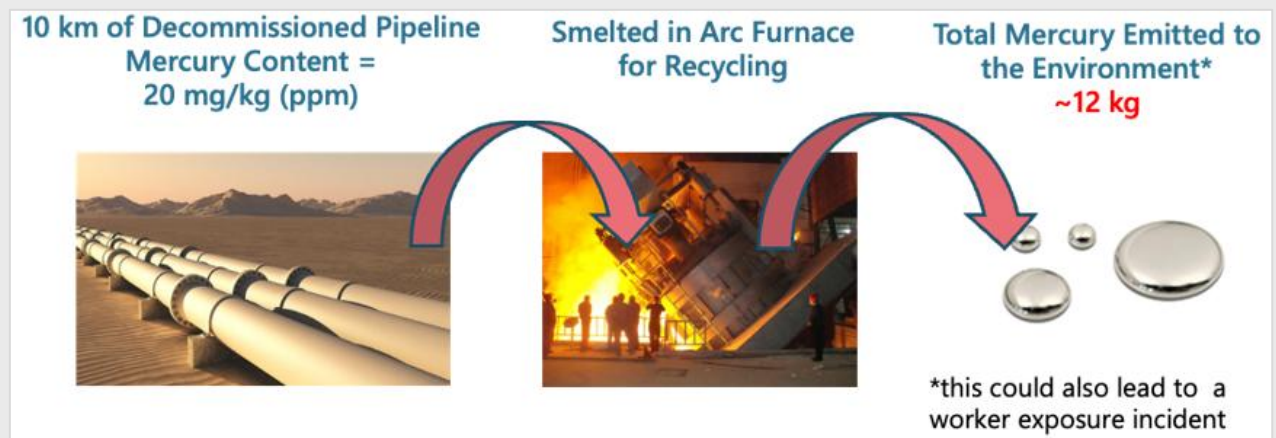
Figure : Pathway for mercury from steel to contaminate steel smelters
