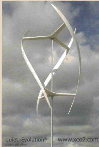
New silent and elegant vertical-axis wind turbine (VAWT), developed by XCO2, winner of DTI SMART award.
