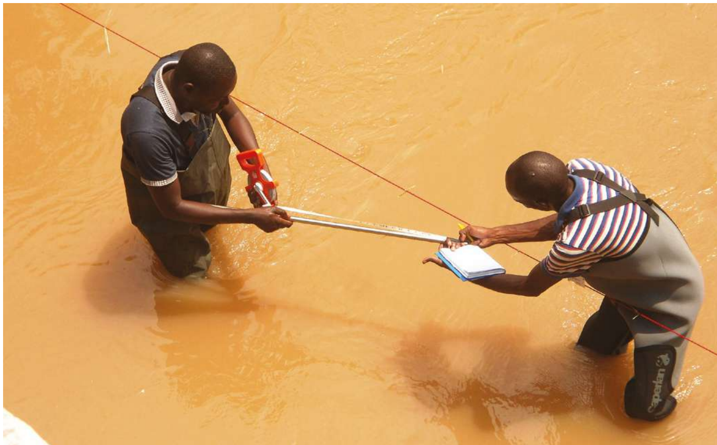
Measuring river flow in Kimwenza
