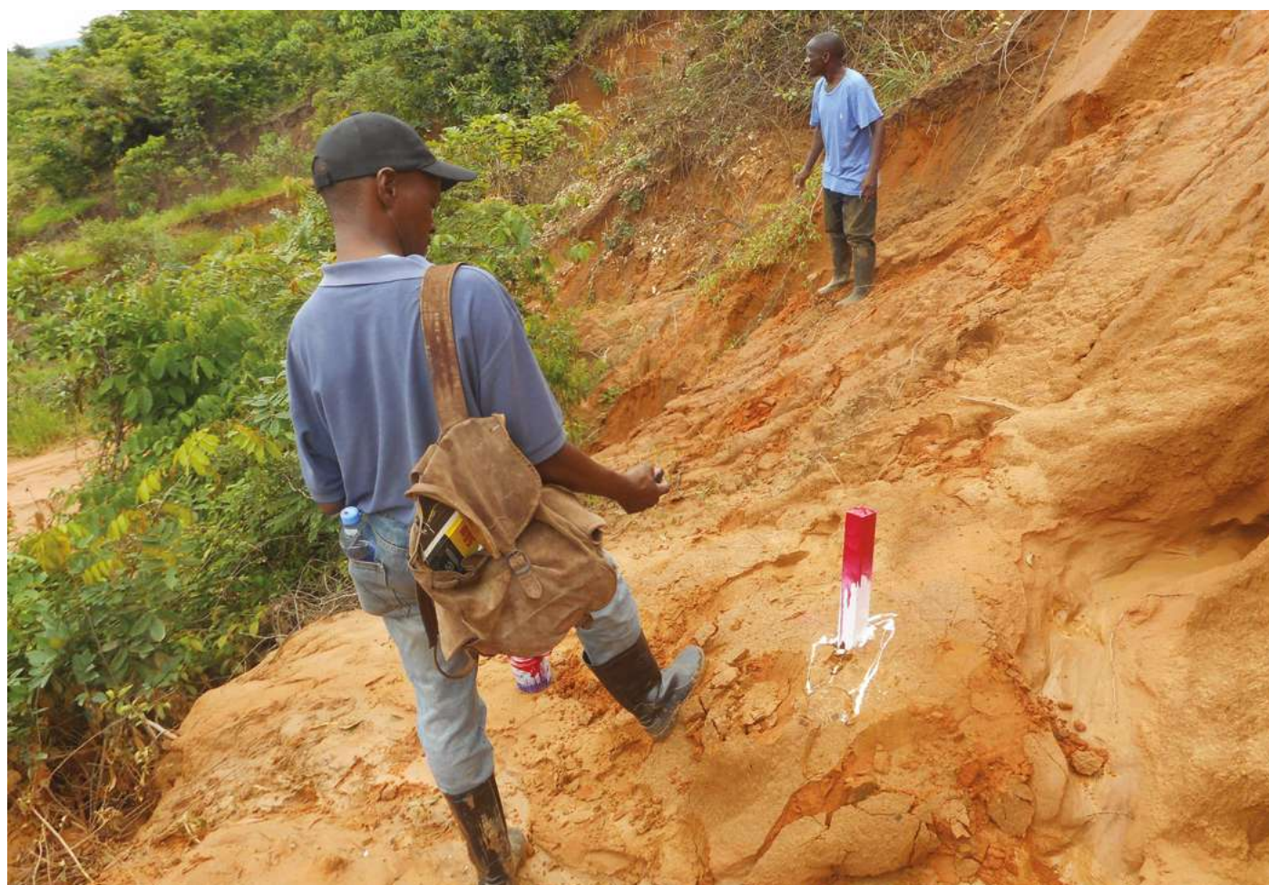
Installation of erosion pins in Mafumba. A total of 110 erosion pins were installed and georeferenced.
