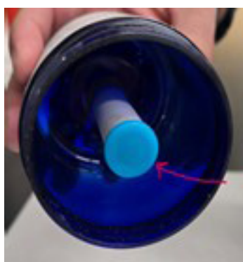
Figure 6. Solid transport lid used for storage prior to deployment (blue arrow)
