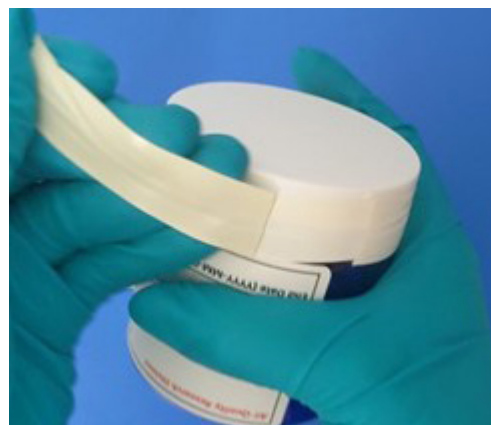
Figure 8. Example of labelling of Merpas® sample and blank units prior to deployment.
