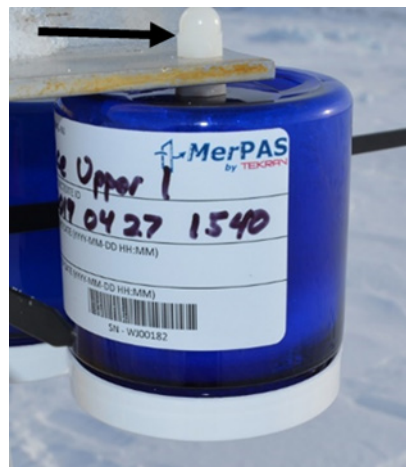
Figure 14. Removing the Merpas®.
