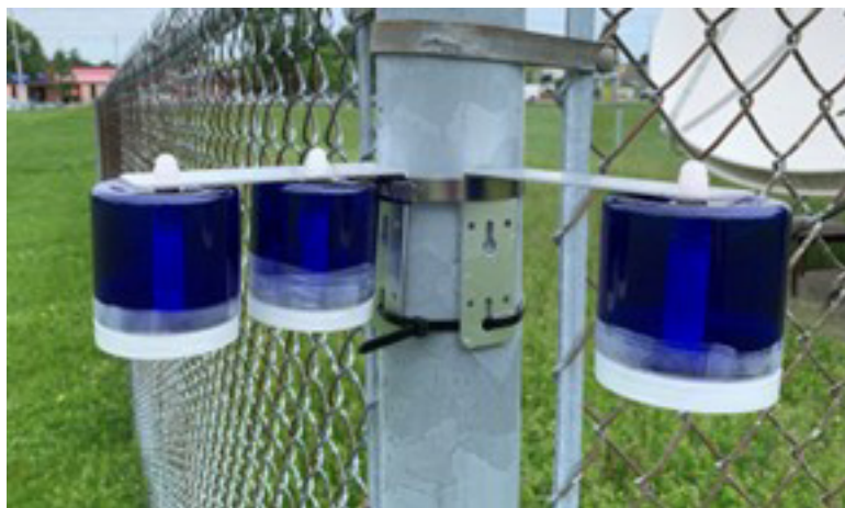
Figure 4. MerPAS® samplers mounted on a pole for field deployment
