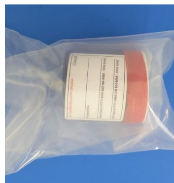
Figure 18. Placement of field blank and sample units in ziplock bags (double bagged).
