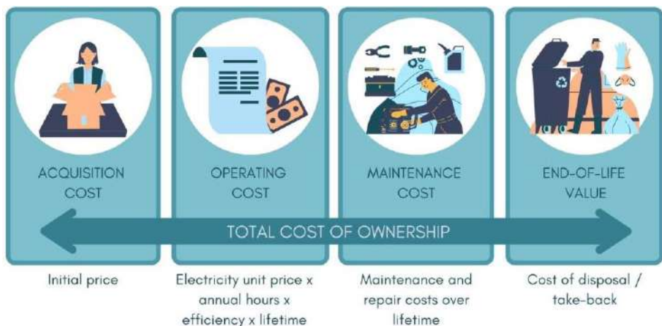
Figure 18: Calculating Total Cost of Ownership (TCO) for a Room Air Conditioner
