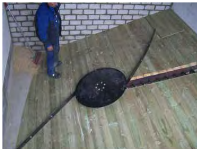
Figure 3: Typical Sweeping Floor System
