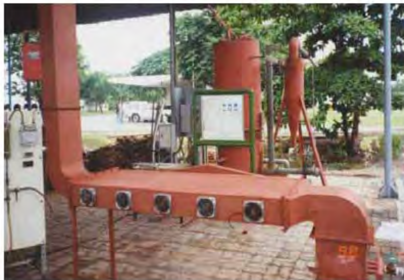
Figure 3.3: Biomass stove-heat exchanger unit without insulation
