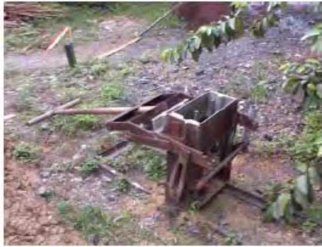
Fig. 4: a) Hand press used for the SFB manufacture, b) Discarded CINVA-RAM press
