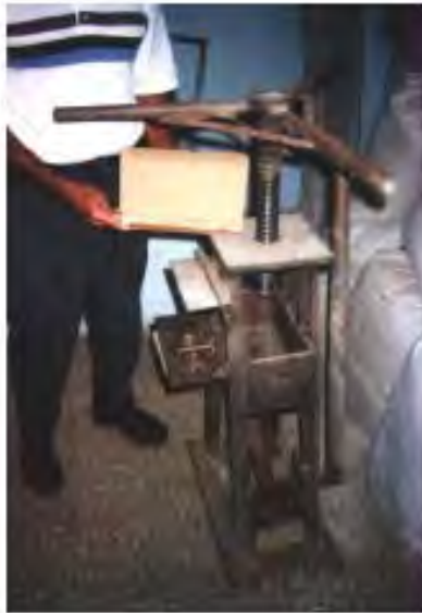
Fig. 4: a) Hand press used for the SFB manufacture, b) Discarded CINVA-RAM press
