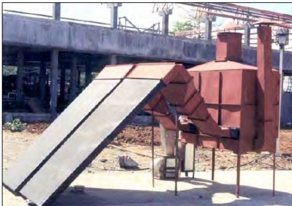
Figure 10.4: The transpired collector solar-biomass hybrid cabinet dryer
