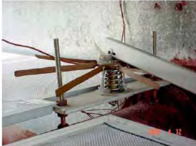
Figure 2.19: Thermostat used in the temperature control mechanism
