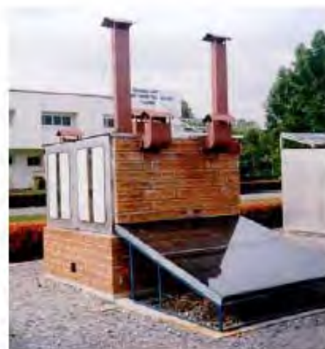
Figure 2.2 Solar-biomass hybrid cabinet dryer
