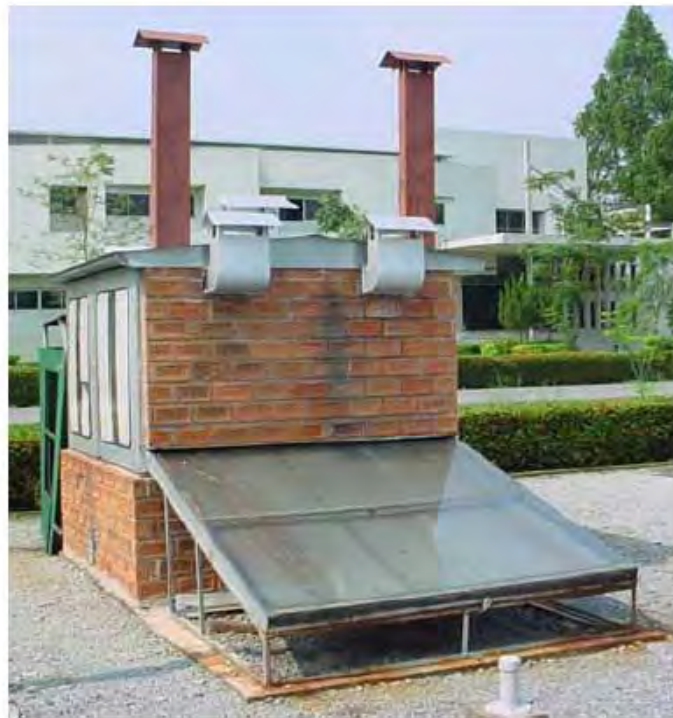
Figure 2.20: The solar-biomass hybrid cabinet dryer
