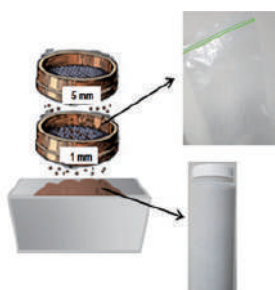
Figure 6: A simplified diagram of sieved fractions and sample collection
