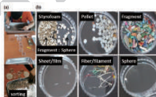
Figure 7: a) Visual Quantification of L-MP in the laboratory, and b) plastic's
