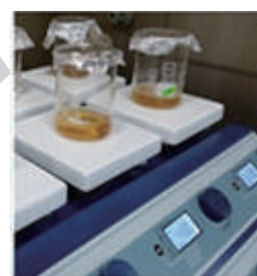
Figure 9: Beakers on magnetic stirrers in a fume hood during removal of organic matter
