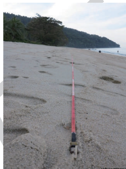
Figure 2: Marking a 100 m stretch on a selected reference line
