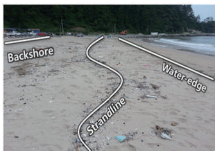
Figure 1: The referent lines for beach sediment sampling
