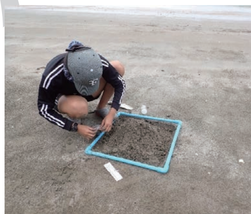
Figure 4: Placing a 0.5 m x 0.5 m quadrat on a beach for MP sample collection
