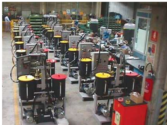
Specially designed low-cost foam dispensers for the first SME group project in India.
