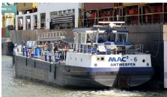
Barge collecting liquid oily waste (Photo credits: MAC² Antwerp, Belgium)
