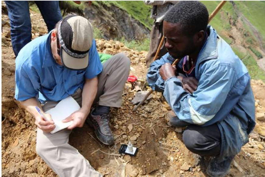
Mercury inventory using an electronic balance to measure ratio of mercury loss to gold produced, UNEP.
