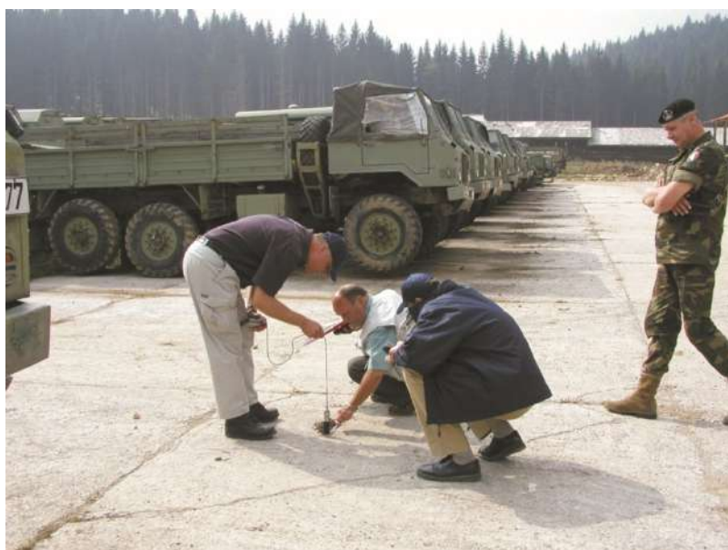
Beta radiation measurements during the pre-mission helped identify contamination spots, 2002, UNEP.
