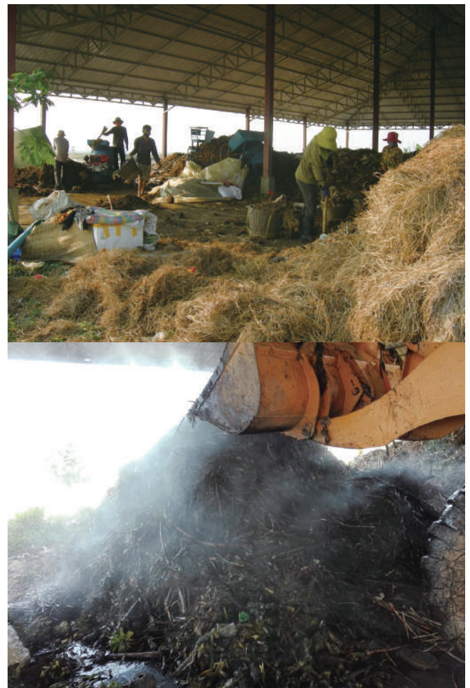
Figure 12: Windrow Composting of Organic Waste
